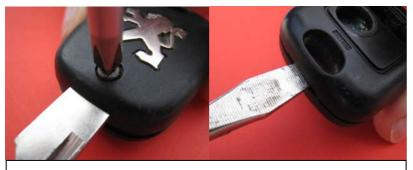
Use Phillips screwdriver to unscrew remote and prise it open on the split line.
