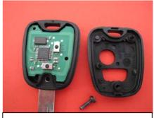
Once you open your remote you end up with bottom part consisting electronics and top part with plastic button shell.
