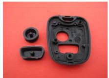
Using a hobby knife, carefully trim the old worn buttons from the plastic key casing.
